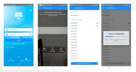
3. After entering the APP, select the "Console" menu, click the "Hybrid Setting" option, click "Other" under the "Generator" option, and check the "parallel Mode" to activate parallel mode.
