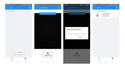
4. Click the inverter in the Plant to enter the monitoring interface of that inverter.
