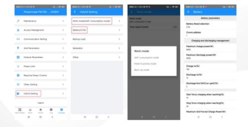
6. "The time-based Control" of the inverter can be activated in the "Work mode" setting.
