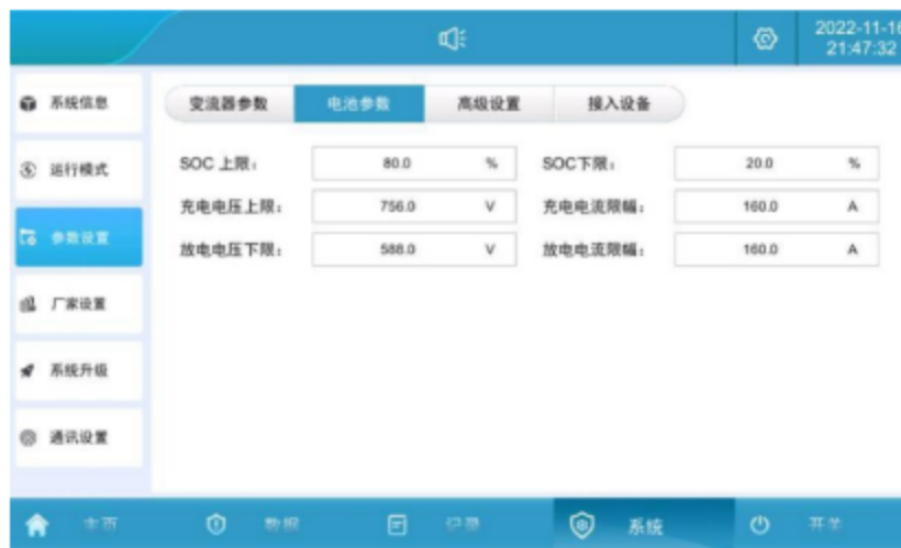
Figure 5.21 Battery charge and discharge setting screen
