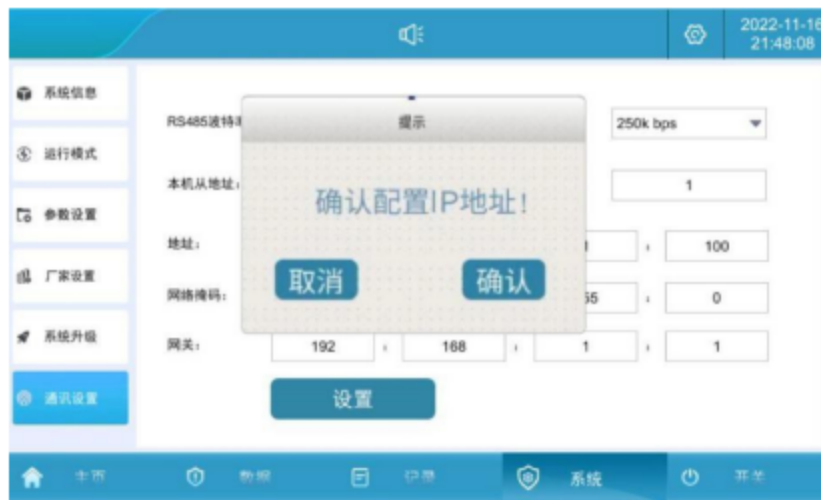
Figure 5.8 IP Address configuration interface
