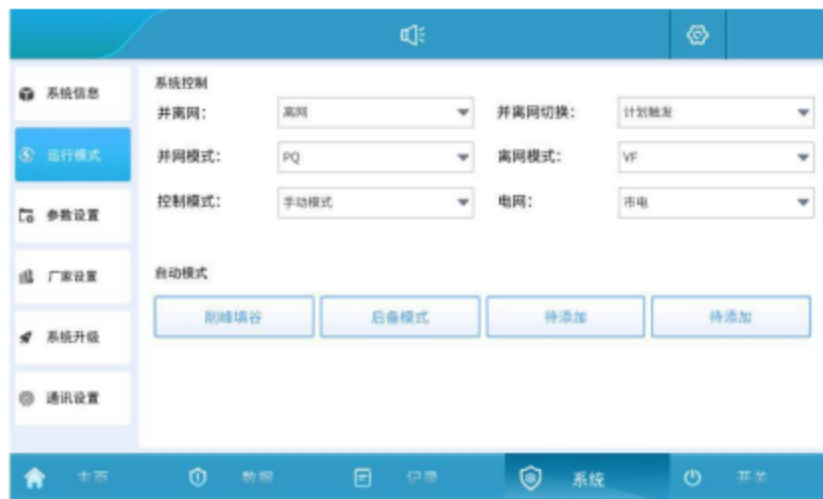
Figure 5.19 Manual and off-network switching mode setting interface
