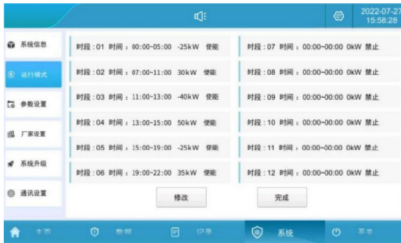
Figure 5.13 Charge and discharge setting interface of peak clipping and valley filling
