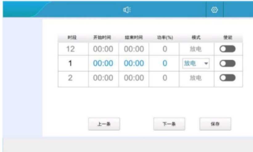
Figure 5.12 Setting interface of charge and discharge time for peak clipping and valley filling
